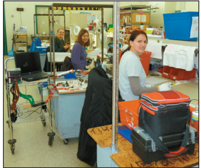
The NRI Data Cell assembling the less complex harnesses. All harnesses are tested using the Cirris Easy Tester on the cart.
